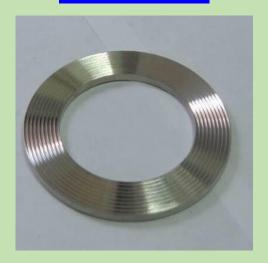
Stoplick serrated gaskets are designed for high pressure, high temperature or highly corrosive applications by Selecting the most suitable materials and shapes. It can be used without sealing layers to provide an excellent sealing but there is a risk of flange surface damage especially at high sealing pressure.
